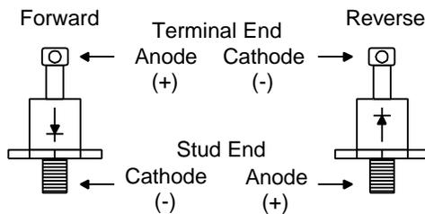
FIGURE 3: DIODE POLARITY
